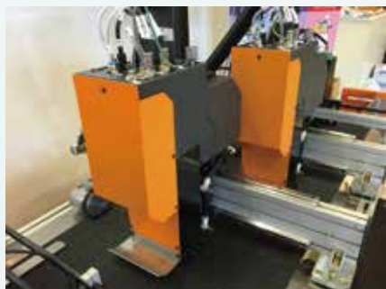
Print Head Modules Mounted on Supports
